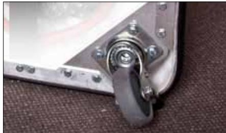
Four omnidirectional castors makes moving the machine on the job or transporting, smooth and easy. With one lockable wheel as a brake, 'Terminator' is 100% stable as well as easy to use ...and move.
