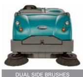
Achieve outstanding results in diverse environments with dual side brushes which allows you to sweep a path of 2,032 mm in a single pass.
